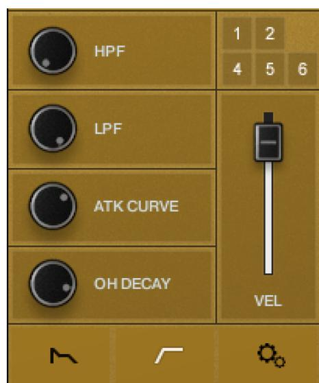
**HPF:** A high pass filter, which removes low frequencies from the sound.
