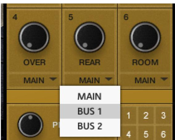
Each drum features 3 stereo ambient / room mic controls. You can choose to route these either out through the same channel as the other mics for that drum ('drum channel'), or through one of two assignable Bus channels. In this way you can have a traditional 'Overheads' or 'Room' channel if you wish to process all mics together.
