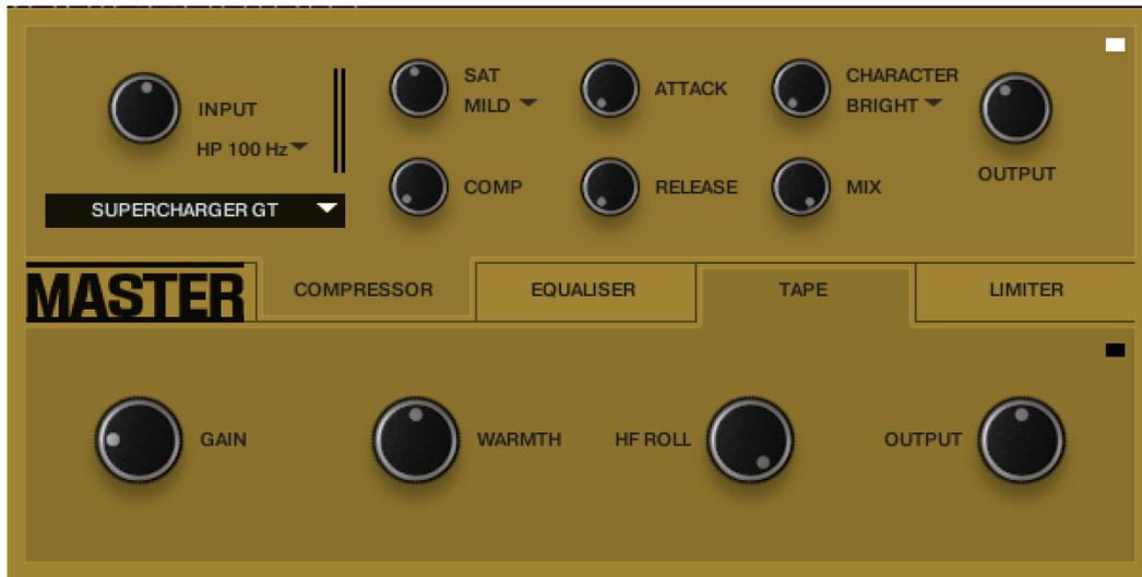
**COMPRESSOR:** This can be switched between Supercharger GT, Feedback Comp and Bus Comp (SSL) mode. All 3 have a MIX control for parallel compression techniques. Only one can be active at once.
