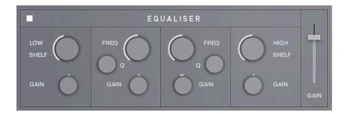
Note that BELL and SHELF are drop down menus, you can choose either for the top and bottom bands. You can enable or disable the EQ with the power switch at the top left.
