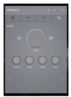
The LFO tab lets you control the LFO RATE, as well as the depth of modulation to the PITCH, AMPlitude, FILTER cutoff or PAN of that department.
