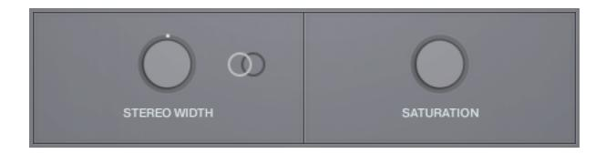
Here you can adjust the STEREO WIDTH (the natural recording is nominal at 12 o'clock). Moving the control left narrows the width, and to the right increases it.
