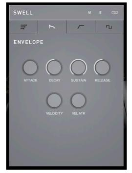
The ENVELOPE tab gives you control of the ADSR Amplitude envelope, as well as VELOCITY sensitivity and VELOCITY to ATTACK time modulation depth.
